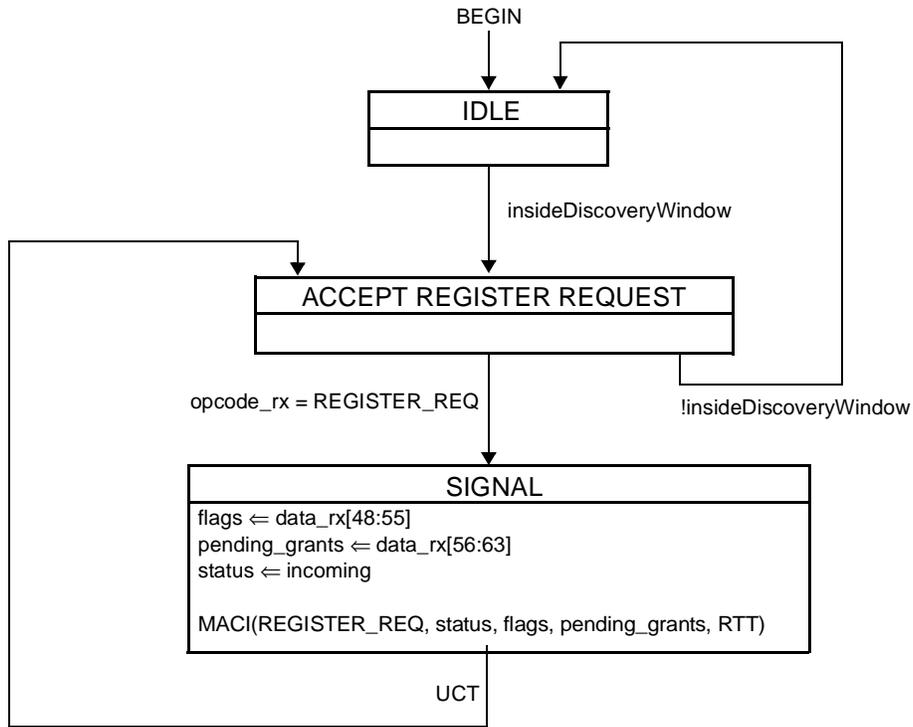
Figure 64–19—Discovery Processing OLT Process Requests State Diagram
