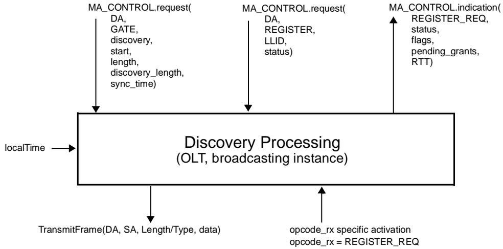
**Figure 64–15—Discovery Processing Service Interfaces (OLT, broadcasting instance)**
