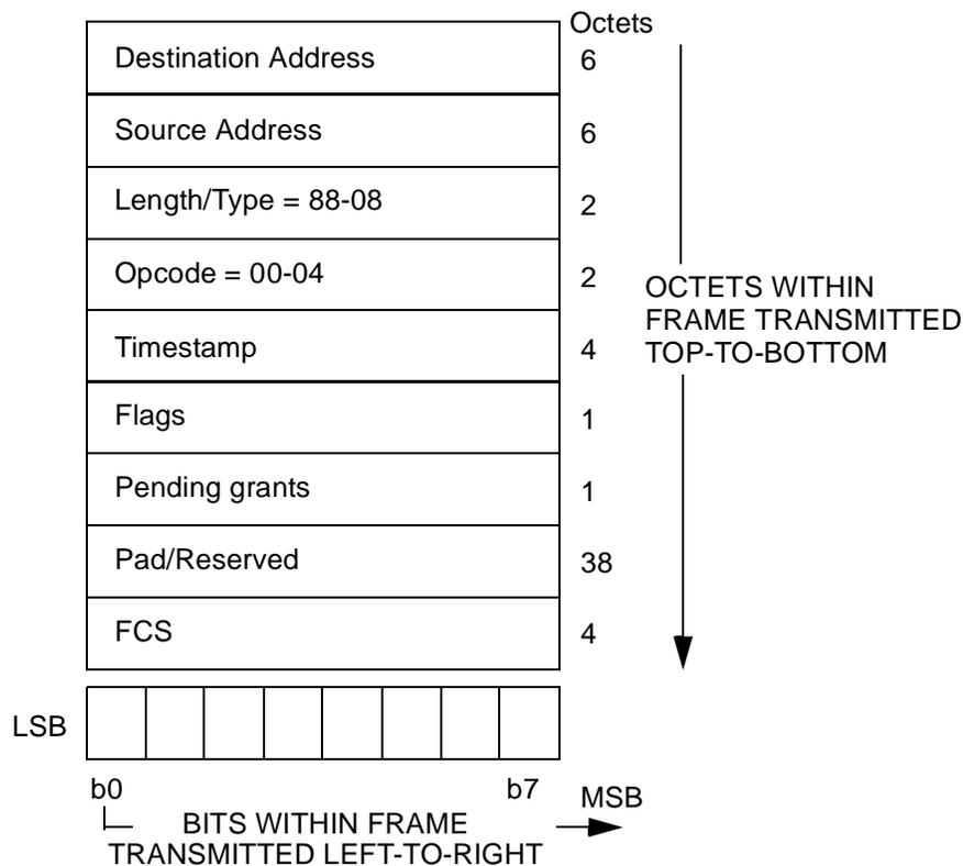
**Figure 64–33—REGISTER\_REQ MPCPDU**
