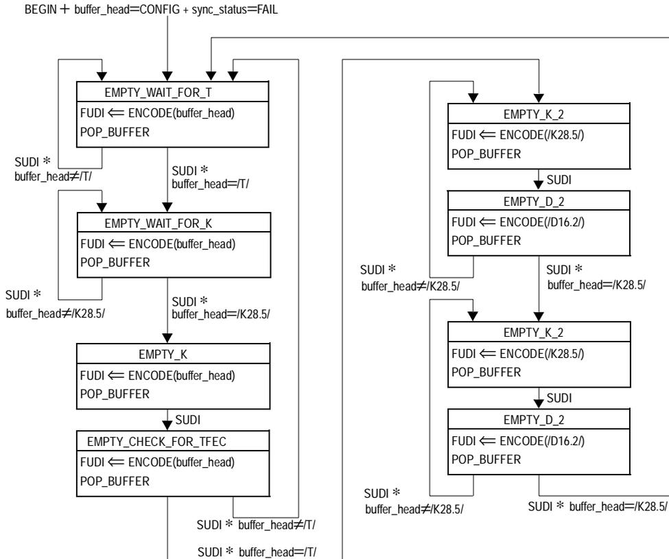
**Figure 65–14—Receive buffer-empty state diagram**
