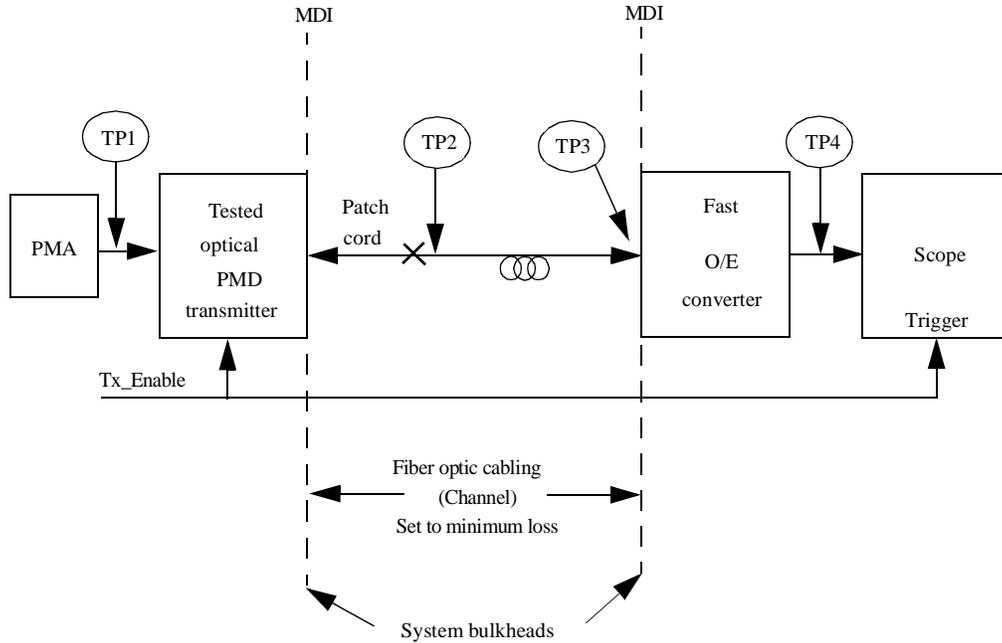
**Figure 60-8—ONU PMD Laser on/off time measurement setup**
