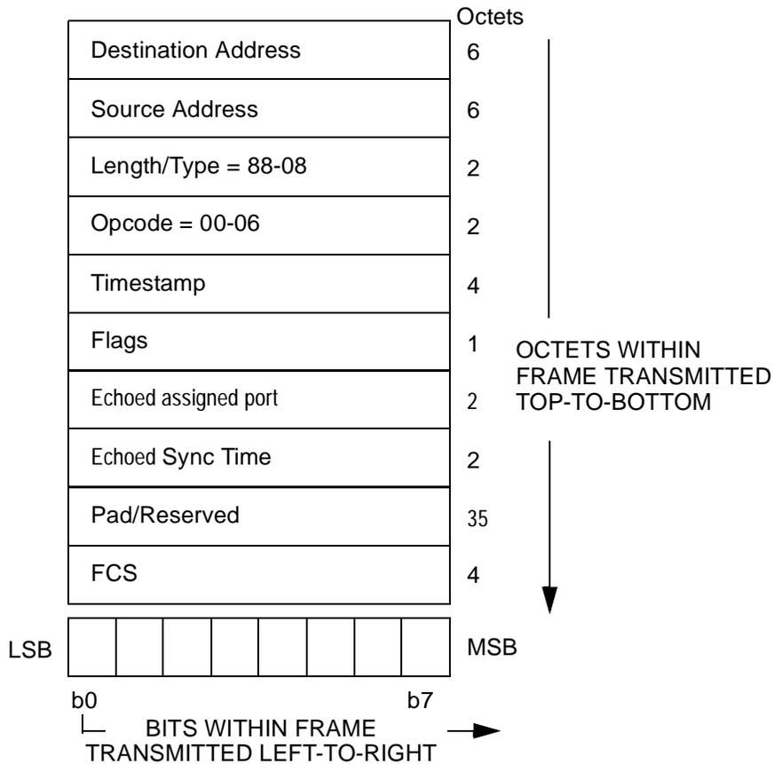
**Figure 64–35—REGISTER\_ACK MPCPDU**
