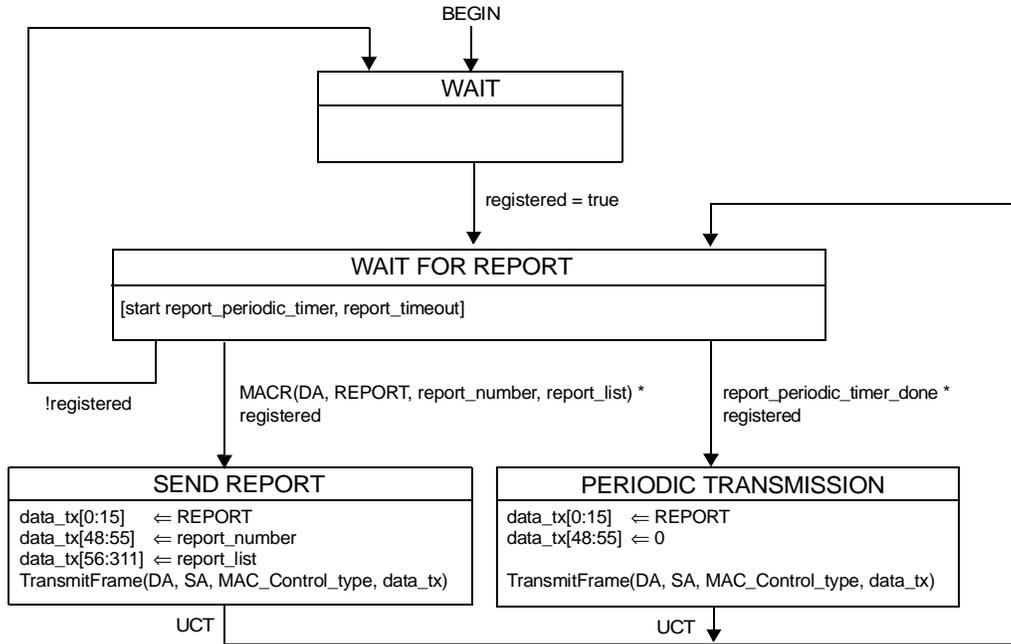
**Figure 64–25—Report Processing State Diagram at ONU**
