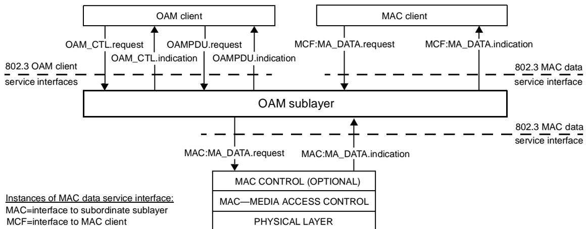
Figure 57–2—OAM sublayer support of interlayer service interfaces
