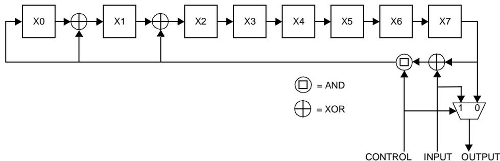
CONTROL = 1 when shifting the modified preamble and calculating the CRC
