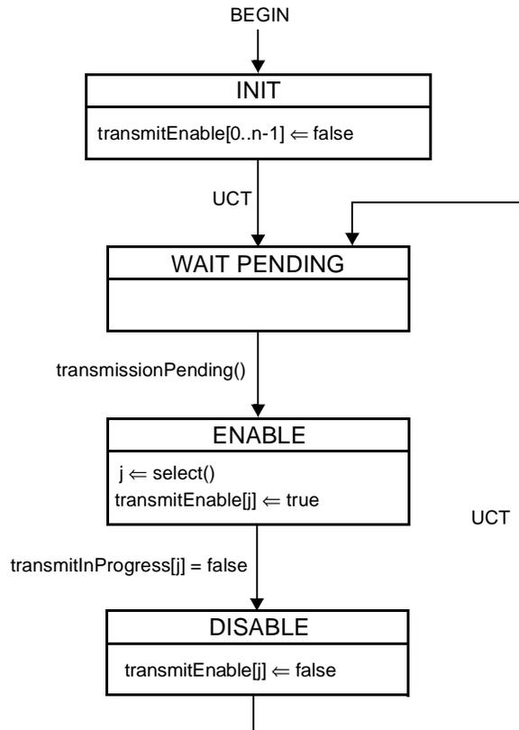
Figure 64–9—OLT Multi-Point Transmission Control state diagram
