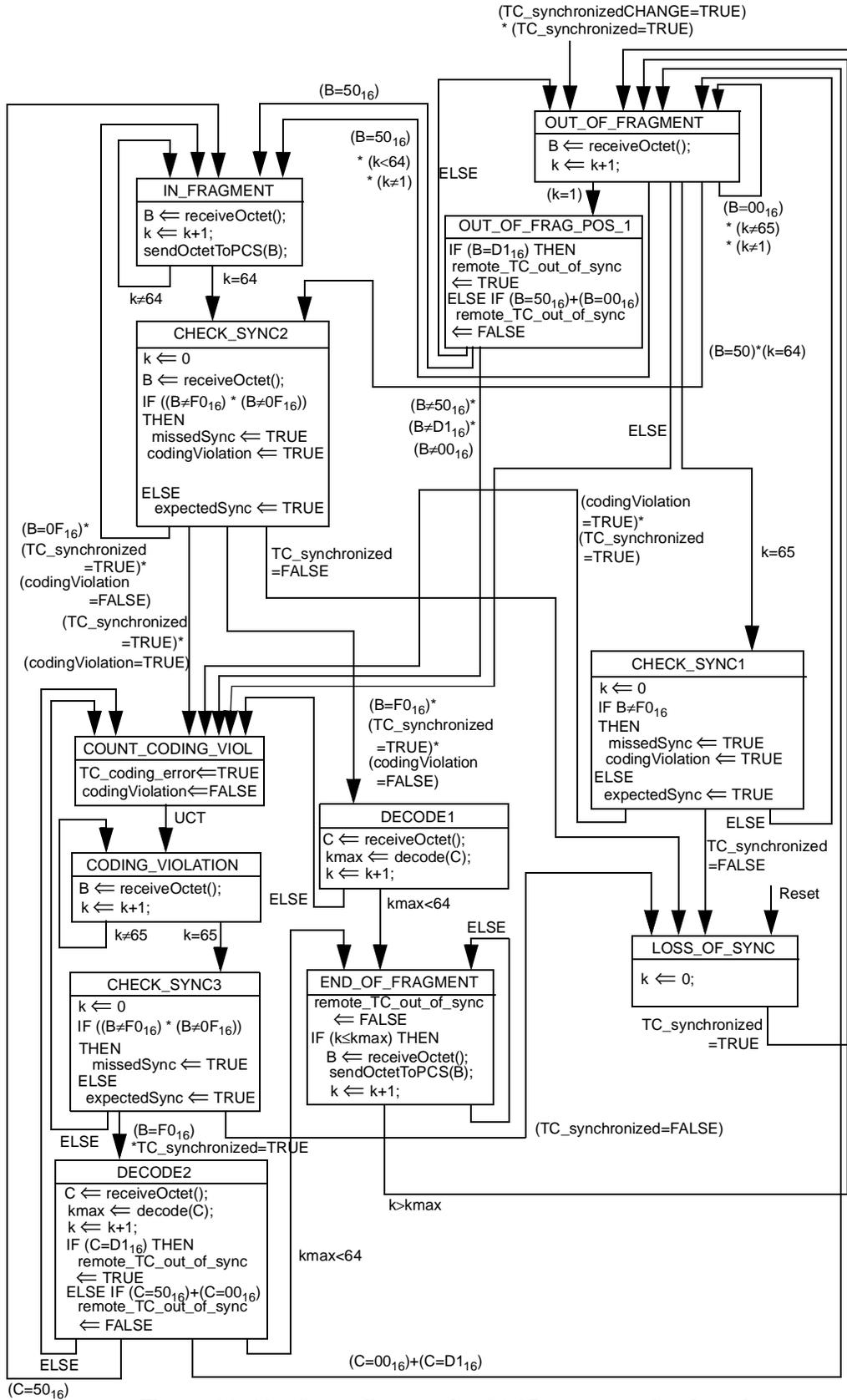
Figure 61-19—State diagram for 64/65-octet receive function
