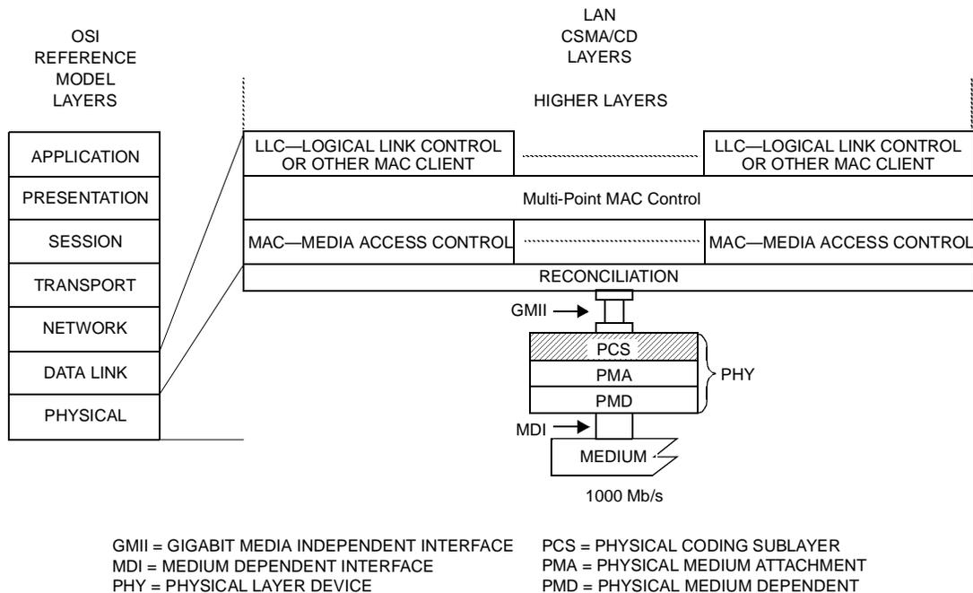
**Figure 65–3—PCS location in the OSI protocol stack**
