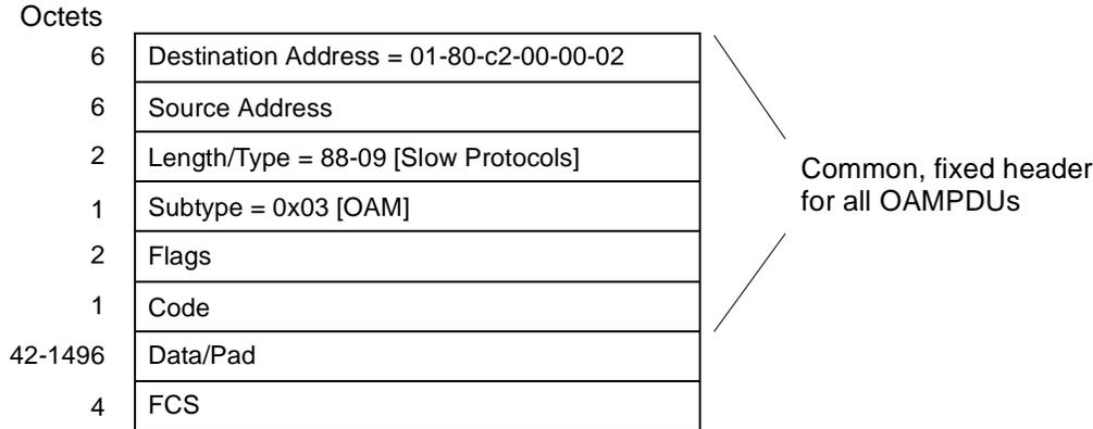
**Figure 57–9—OAMPDU frame structure**
