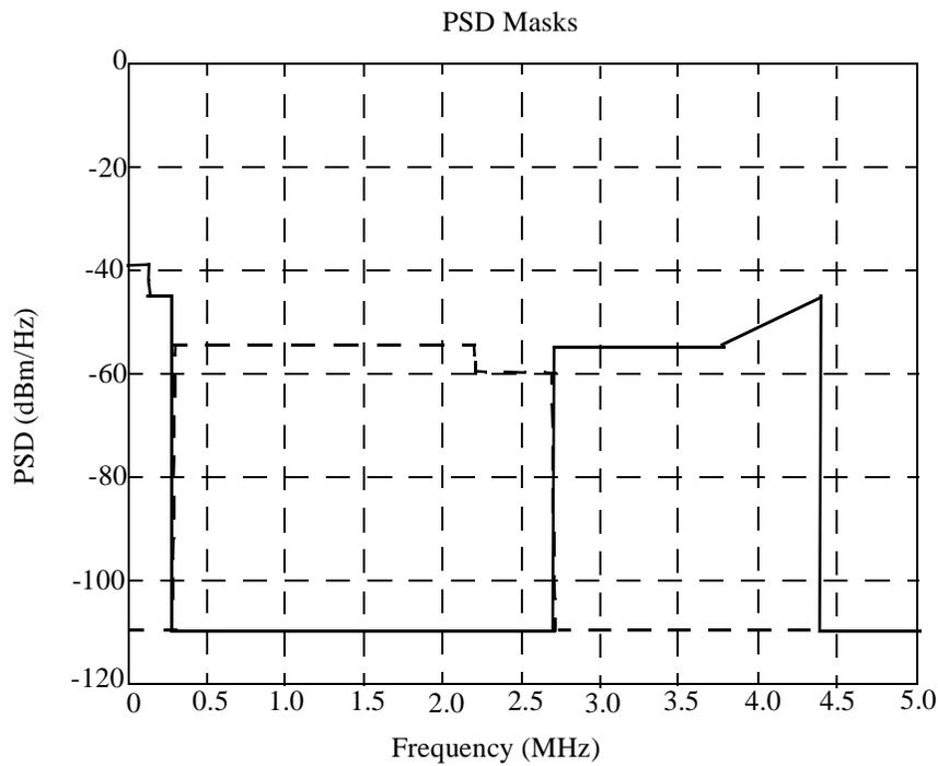
**Figure 62C-1—Example PSD Masks for MCM 10PASS-TS**
