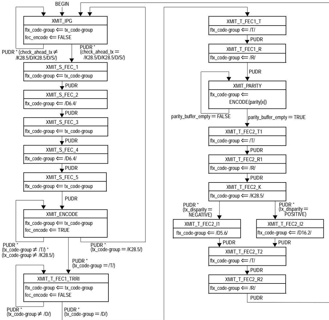
Figure 65–11—Transmit state diagram
