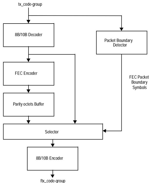
**Figure 65–8—Transmit block diagram**
