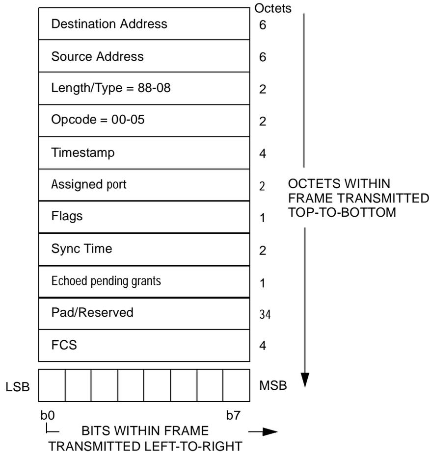
**Figure 64–34—REGISTER MPCPDU**
