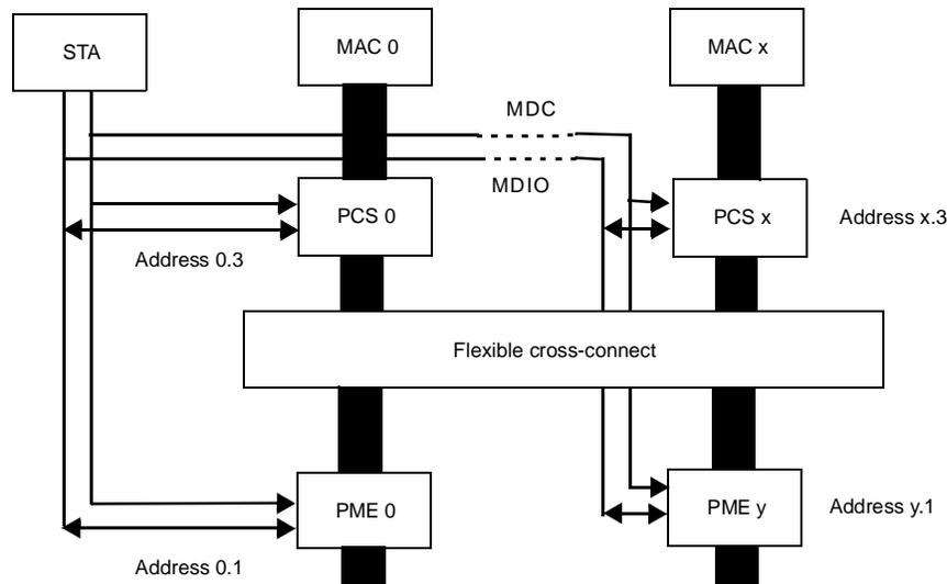
Figure 61–3—Connection of MDIO bus to MMD instances
