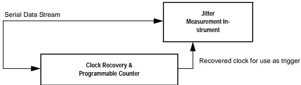
Figure 59–5—Utilization of clock recovery unit during measurement
