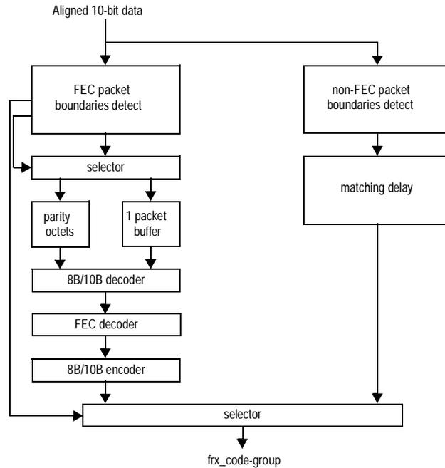
**Figure 65-10—Receive data block diagram**
