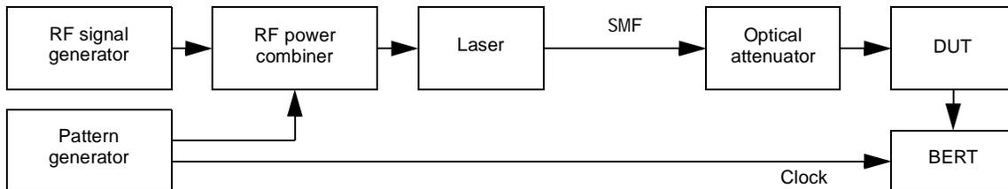
**Figure 59–6—Test setup for receiver bandwidth measurement**
