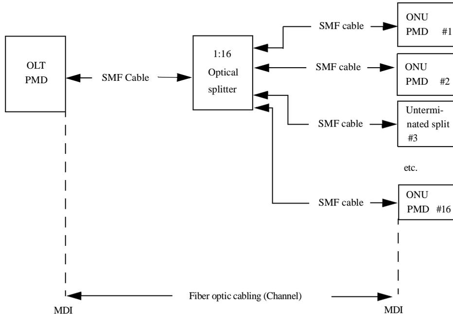
**Figure 60–10—Fiber optic cable model**
